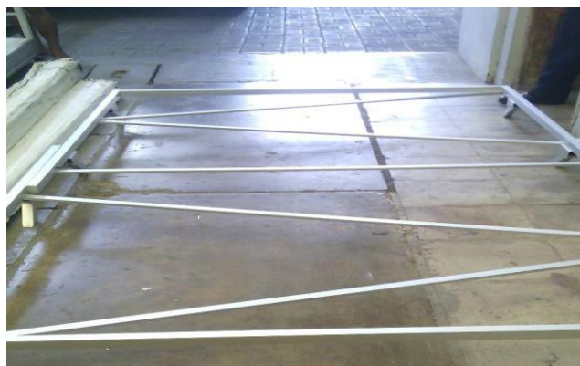
Figure 1: Batik ciprat frame made of stainless steel
