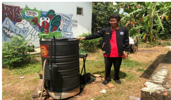
Figure 2. Apparatus for Distilling Plastic Waste into Liquid Fuel (BBM)
